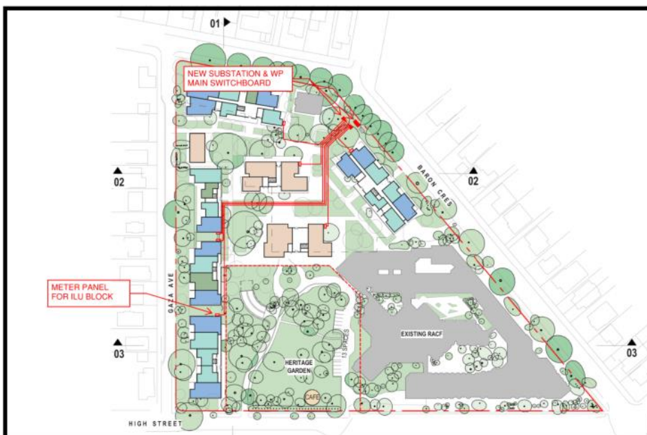
Figure 5.2 Proposed LV reticulation to new ILU Buildings
